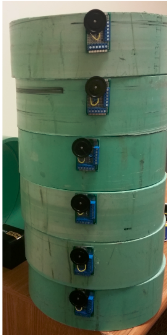
Figure 15: Circuit boards glued to inductor rings (jigs)
